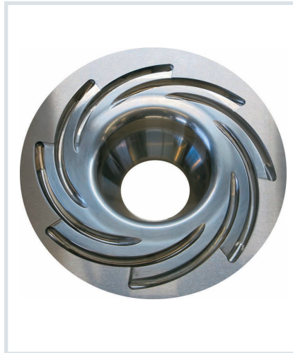
Fig. 1. The circular distribution principle: left: a circular distributor, right: the simulation of radial circumferential distribution after pre-distribution of the melt (© ETA)
